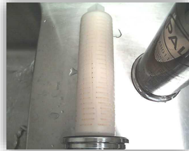
Figure 12 Rouge discolouration found on a point of use 0.45 \mu\text{m} filter
